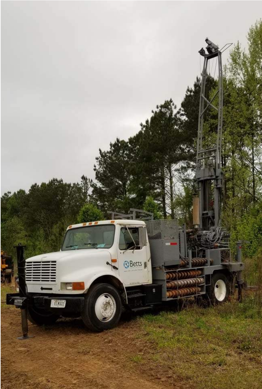
Figure 1: SPT drill rig.
